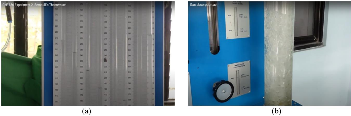
Figure 1. Screenshot taken from (a) Bernoulli theorem video experiment: water levels in the columns; and (b) Gas absorption video experiment: packed tower columns.
